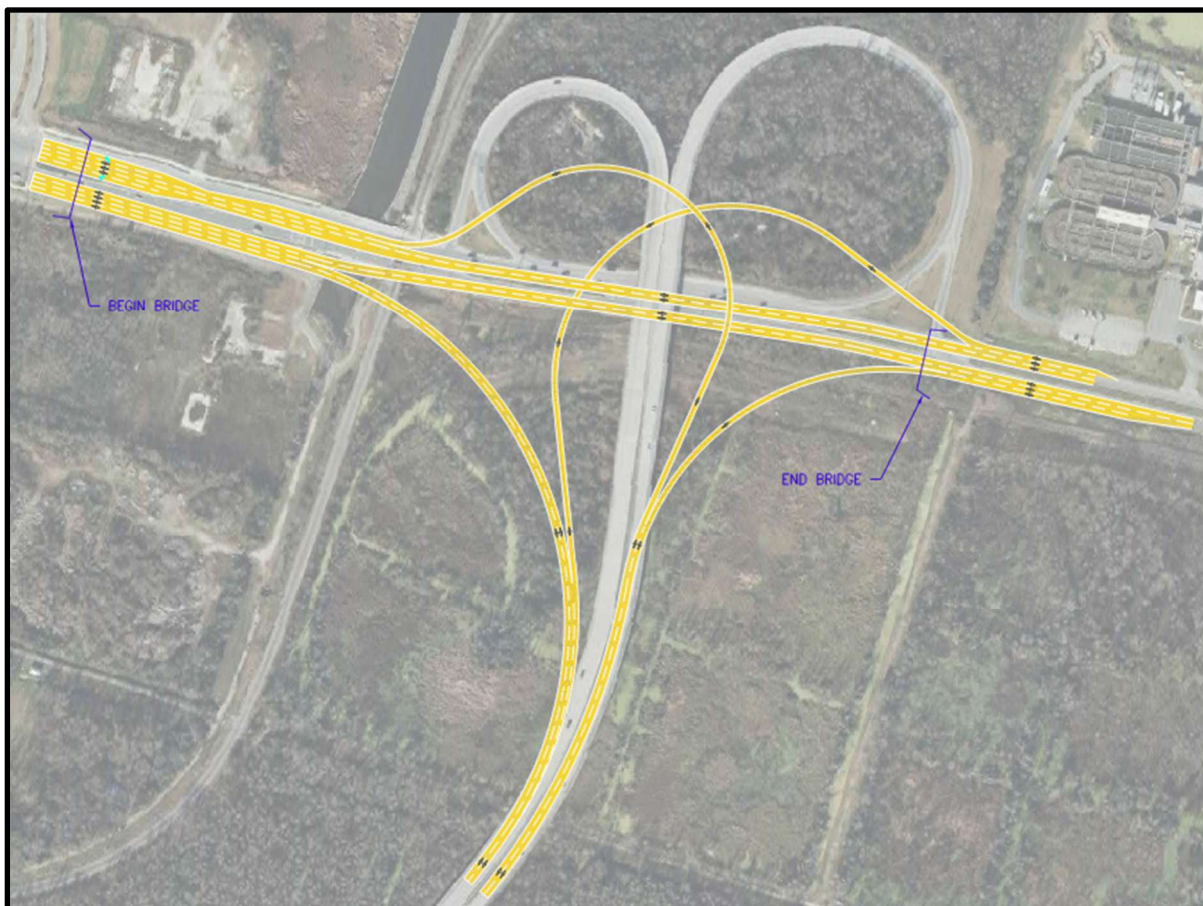
Figure 25: Alternative 6 – Free-flow Flyover Interchange
